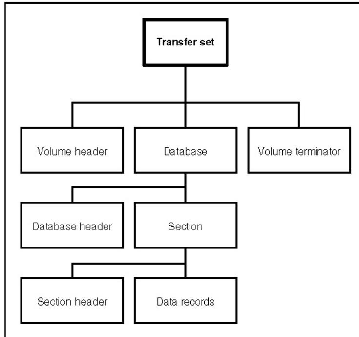
Figure 5.2: Physical file structure of an NTF file
