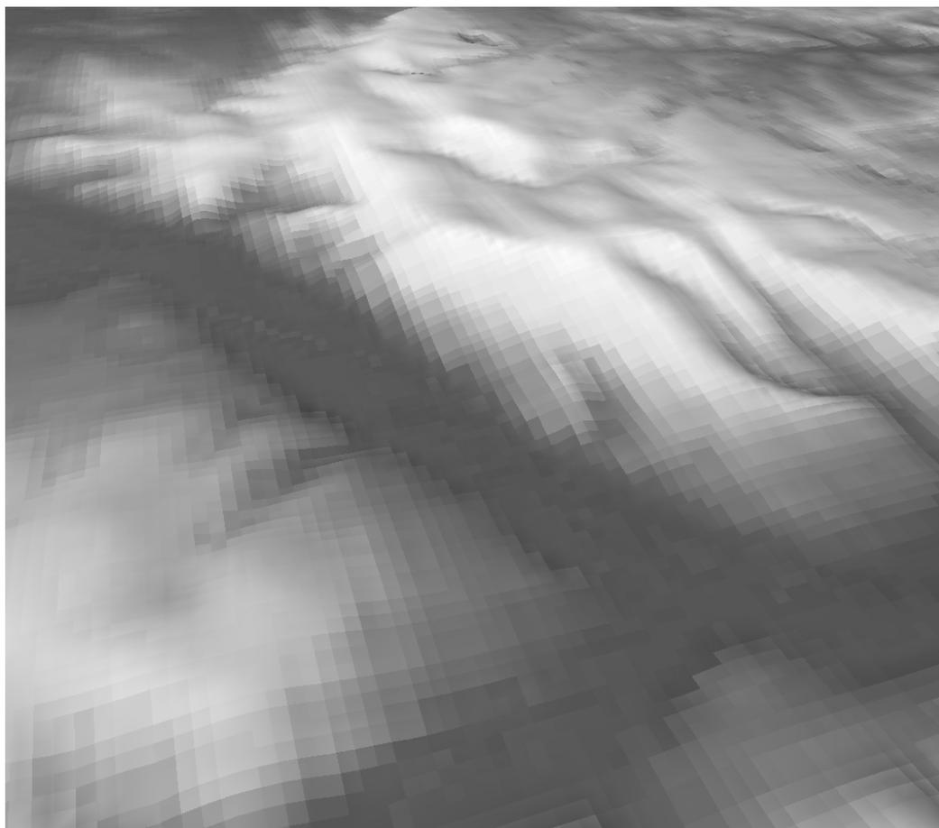
OS Terrain 50 posts displayed as a heightened, shaded raster in a GIS.
