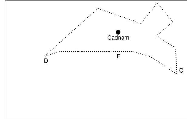
The common line (D–E) to the A31(T) and the settlement polygon, and the common line (E–C) to the A36 and the settlement polygon, each represent two lines. The geometry of each feature is stored separately in the data.
