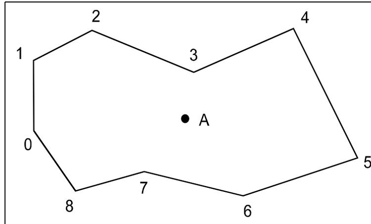
*Point A is the polygon seed point for the area; attached to this point will be attributes, such as the feature code, which define it, and its definitive name – if it is named on the map. The polygon in this example comprises nine individual line segments.*
